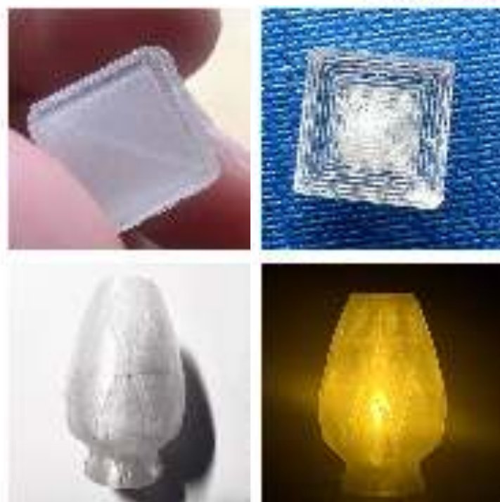
Figure 50. PETG printing test to get transparent layer
