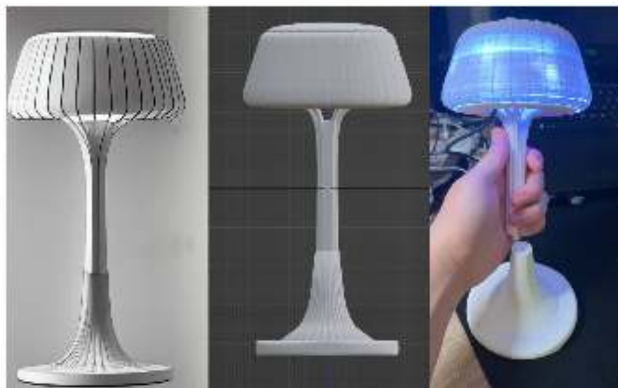
Image / figure 2: the practical applications from 2D AI images to 3D printed lamp models
