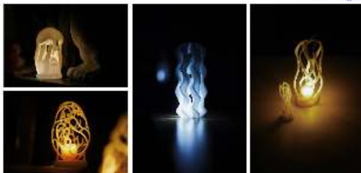
Figure 52. SLA printed lamp covers with white resin
