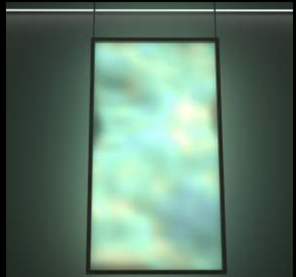
Figure 78: Rendered model of the designed light source. A coded visualisation is mapped to a matrix of LEDs, diffused by acrylic.
