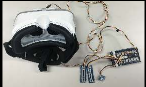
Figure 43: The LED headset and EEG device were used as before, with the addition of sliders to control the frequency and brightness of the LEDs.
