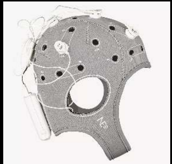
Figure 27: The Enobio 8-channel cap, a typical lab-grade wet electrode EEG device. This particular model was used during this project for all EEG recordings.
